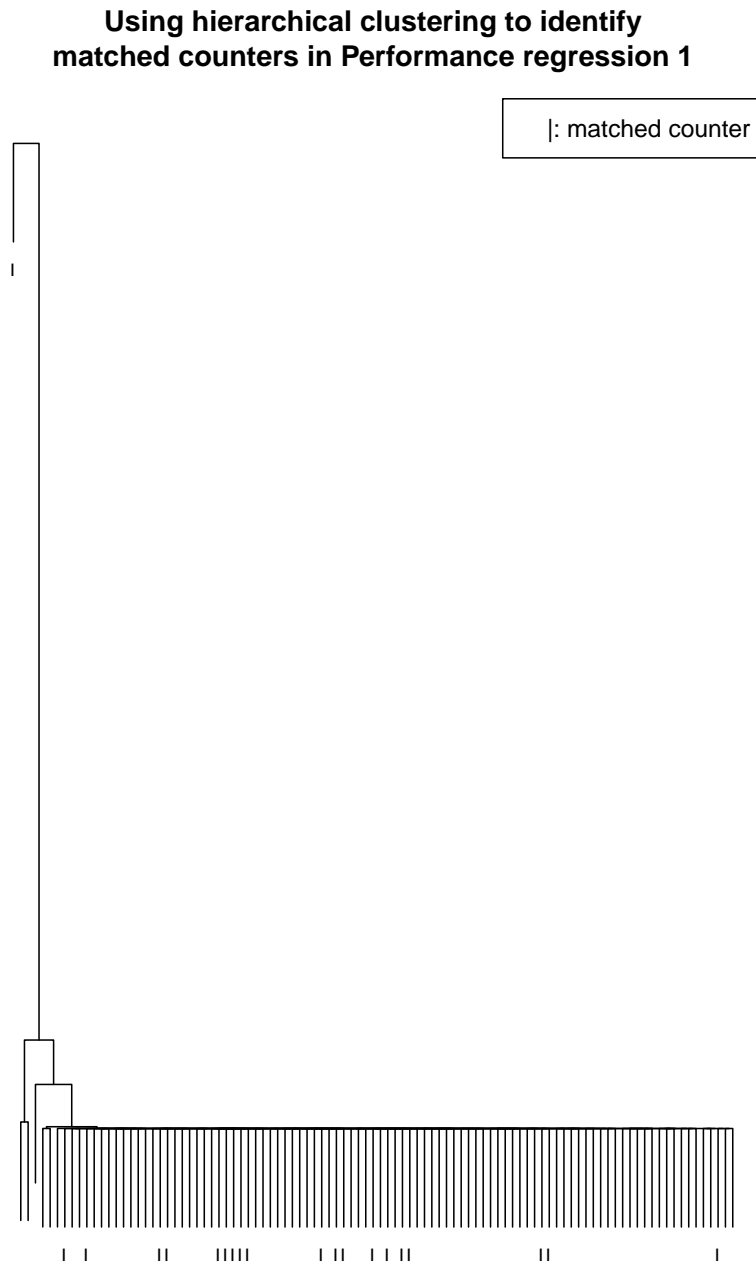
Figure 9.5: Evaluation criterion 2 - Identify the matched counter set using hierarchical clustering for Performance regression 1
