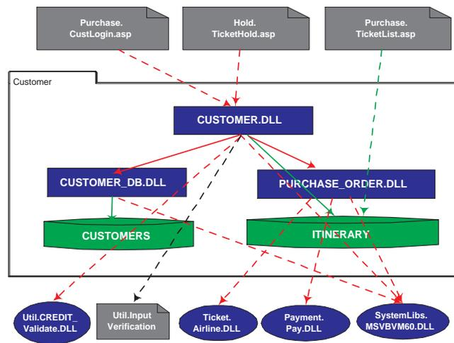
**Figure 6:** The Internals of the *Customer* Subsystem.
