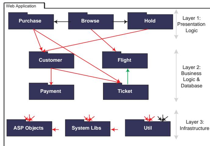
Figure 3: The Recovered Architecture of *Web Flight*.
