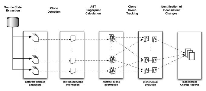
Figure 1. Overview of our approach to study inconsistent changes of code clones at release level.
