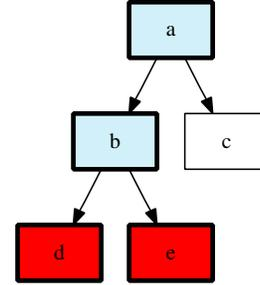
**Figure 4. Change Impact Graph of  $a$  computed using the source code immediately after  $C_3$  but only showing the propagation of the changes  $C_1$  and  $C_2$  (the period of interest includes only these two changes). Red depicts *changed* functions, light blue corresponds to *affected* functions, and white to *unaffected* (*changed* will appear darker than *affected* in black-and-white versions of these images).**
