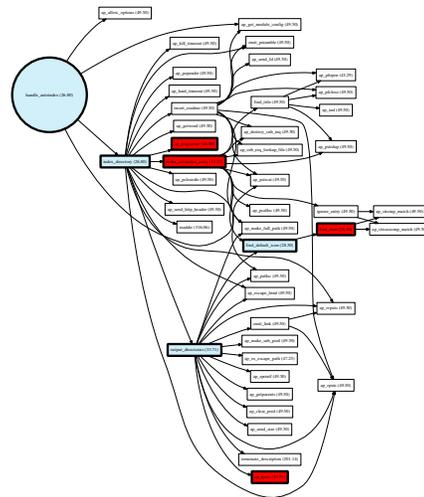
**Figure 7. CIG of `handle_autoindex` on Oct 3, 1998 showing the propagated changes for the last 45 days. The bug was found in the `make_autoindex_entry` function (the second red node starting from the top). For this dependence graph only functions inside the `mod_autoindex.c` file are expanded.**
